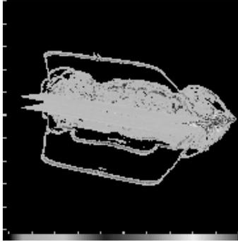
**Figure 4a. Dislocation loops in 35 million atom fracture simulation. (700 Mbytes).**
